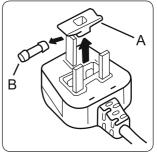
The mains lead of this appliance has been fitted with a BS 1363A 13A fused plug. To change a fuse in this type of plug, follow the steps below:
