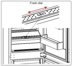
If the crisper is full, the fresh dial located in front of the crisper should be opened. This allows the air in the crisper and the humidity rate to be controlled, to increase the life of food within.
