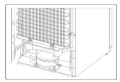
Your appliance performs automatic defrosting. The water formed as a result of defrosting passes through the water collection spout, flows into the vaporisation container behind your appliance and evaporates there.
