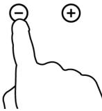
3. While the timer display is flashing, touching the plus and minus keys together returns the time to '00' and cancels the minute minder function.
