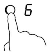
Turn the cooking zone off by touching the minus key repeatedly until the display shows 0, or by touching the plus and minus keys together.
