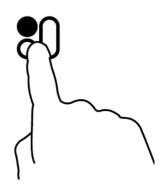
2. While the power level indicator is flashing, touch the fry function key. 'F' appears in the power level indicator to show that zone 2 is currently heating in fry mode. The 'F' indicates that the fry function is active.
