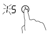
5. While the tens digit is flashing, use the slider control to select the tens digit of the minute minder duration time.
