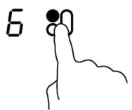
While the power level indicator is flashing, use the slider control to turn the power level down to 0. The zone switches off.
