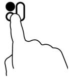
While the power level indicator is flashing, touch the keep warm function key. 'U' appears in the power level indicator display.
