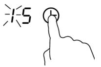
5. While the tens digit is flashing, use the touch control slider key to set the tens digit of the cooking duration time, e.g. 9 in this example to make 95 minutes in total.
