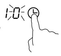
3. While the units digit is flashing, use the touch control slider to set the units digit of the cooking duration time, e.g. 5 in this example.
