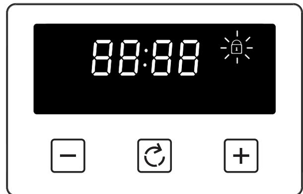
Once the Key lock is active, the buttons will be inactive. A two beep signal will be heard if the buttons are pressed.
