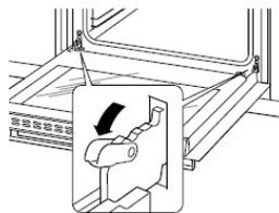
2. Close the door to an angle approximately 30°. Hold the door with one hand on each side. Lift up and slowly pull the door out from the oven.
