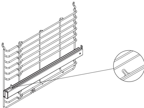
Before removing the shelves completely, please make sure that the shelf is unclipped from the retaining tabs.
