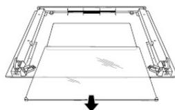
To reassemble, follow the instructions in reverse, ensuring the glass is re-installed the right way up.
