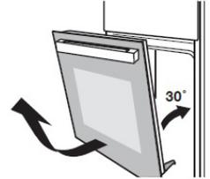
3. Open the door rotation bracket assembly, refer the action in the following picture.
