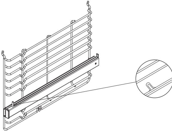
Before removing the shelves completely, please make sure that the shelf is unclipped from the retaining tabs.
