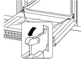
2. Close the door to an angle approximately 30°. Hold the door with one hand on each side. Lift up and slowly pull the door out from the oven.
