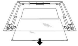
To reassemble, follow the instructions in reverse, ensuring the glass is re-installed the right way up.
