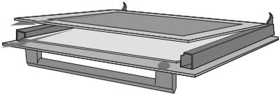
3. Refit the glass in the same order and orientation as removal (Making note of any This Way Up instructions printed on the glass panels)
