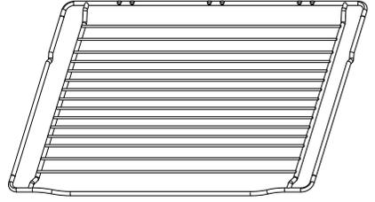
Shelf support rails: Used to support the wire shelf and grill pan if required. These shelf support rails on the right and left sides of the oven can be removed.
