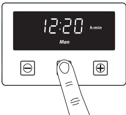
**2** The connectivity symbol will start flashing. The timer is now ready to be connected to a smart device
