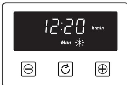
**3** Press and hold the function key for 5 seconds to deactivate the bluetooth connectivity function. The connectivity symbol will disappear.
