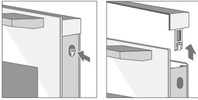
2. Carefully remove the inner glass panels as required for cleaning
