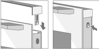
To reassemble, follow the instructions in reverse, ensuring the glass is re-installed the right way up.
