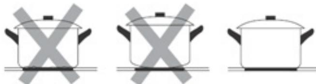
Make sure that the base of your pan is smooth, sits flat against the glass. Use a pan which has a base diameter of at least 145mm. Using a pan which is slightly wider than the glass circle printed on the glass will maximise energy-efficiency. Always centre your pan on the cooking zone.
