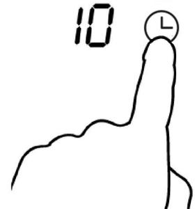
2. While the units figure is flashing, use the power slider to select the units figure of the minute minder duration time (between 0 and 9). Then touch the timer control key again; the tens figure starts to flash. While the tens figure is flashing, use the power slider to select the tens figure (between 0 and 9).
