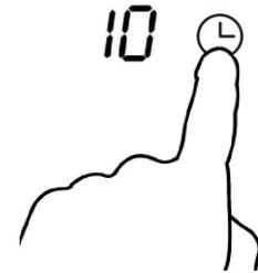
3. While the '0' is flashing, use the power slider to set the units figure (between 0 and 9). Then touch the timer control key again; the '1' (tens figure) starts to flash. While the tens figure is flashing, use the power slider to set the tens figure (between 0 and 9).
