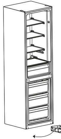
5. Reverse the middle hinge. Screw the middle hinge onto the opposite side of the unit.
