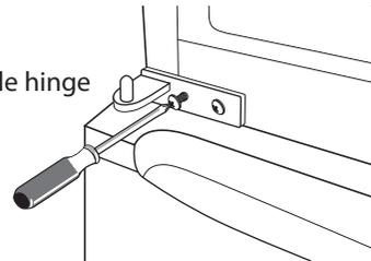
6. Carefully set the upper door back into place, inserting in onto the middle hinge.
