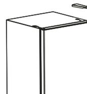
2. Remove the the upper hinge. Lift the upper door and place it on a padded surface to prevent it from scratching.
