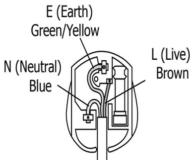
The wires in the mains lead are coloured in accordance with the following code:
