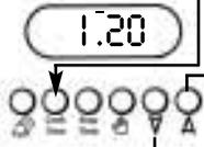
Within 2 seconds press and hold the "▲" button until the required cooking period is set.
