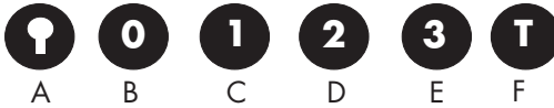
Figure 2: hood controls: The controls work as follows: A - Neon light B - Off C - Position 1 D - Position 2 E - Position 3 F - Light switch
