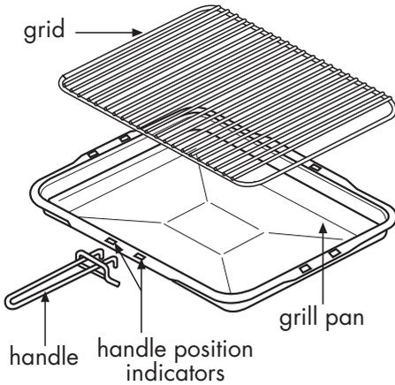
Place the handle over the edge of the grill pan, at the narrow side edges. Slide the handle to the centre, and locate between the handle position
