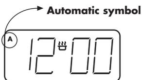
This 'A' symbol appears when either a semi, or fully automatic program is selected. This symbol will flash while a program is being set. Once a program is set the symbol will light up, and remain lit until the alarm sounds, or the program is cancelled
