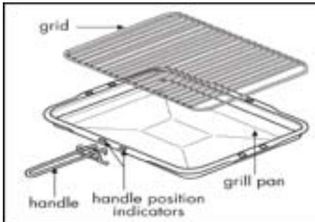
Place the handle over the edge of the grill pan, at the narrow side edges. Slide the handle to the centre, and locate between the handle position.
