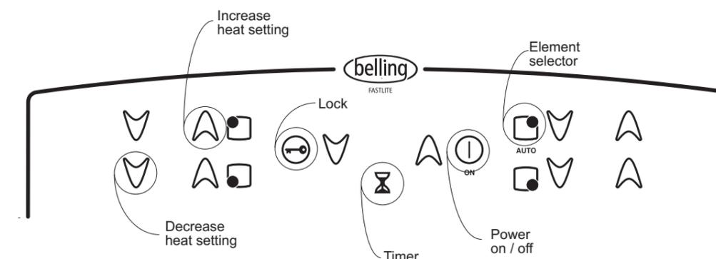
When the hob is first switched the controller will illuminate parts of its displays, accompanied by a beep. This is the controller testing and calibrating itself. When this process is complete the neon adjacent to the lock pad will light, to indicate the hob is ready for use but locked for safety.
