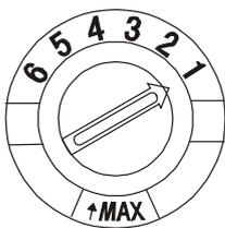
A measured amount of rinse aid is released during the final rinse. As with detergent, the amount of rinse aid needed for your dishes depends on the hardness of the water in your area. Too much rinse aid can result in lather or foaming and cause cloudiness or streaks on your dishes. If the water in your area is very soft, you may not need rinse aid. If you do, you can dilute the rinse aid with an equal amount of water.
