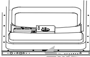
To clean the edge around the door, you should use only a soft warm, damp rag. To prevent penetration of water into the door lock and electrical components, do not use a spray cleaner of any kind.
