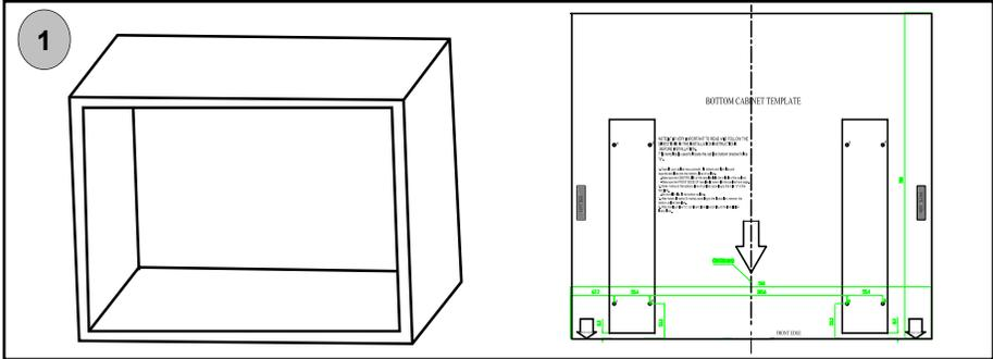
1. Read the instruction on the **BOTTOM CABINET TEMPLATE**, put the template on the bottom plane of cabinet.
