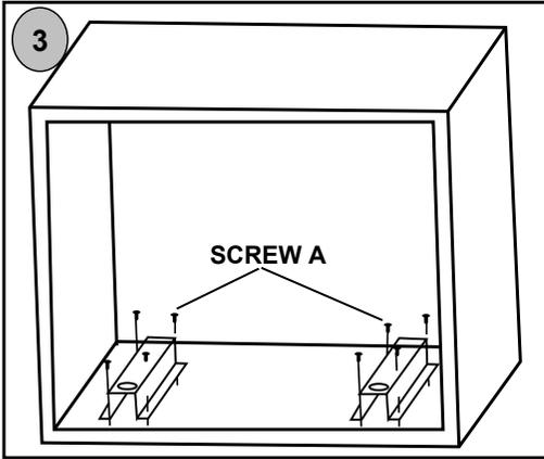
3. Remove the BOTTOM CABINET TEMPLATE, and fix the BOTTOM BRACKETS with SCREW A.
